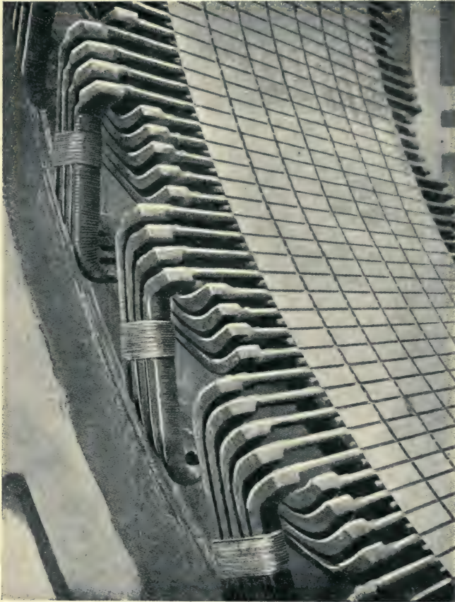
FIG. 398.—Portion of Armature Core and Bar Winding of Westinghouse Alternator.
